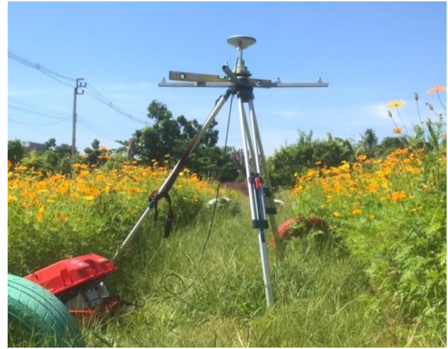
Fig. 13. Testing between Leica Receivers and Low-Cost RTK Receivers.
