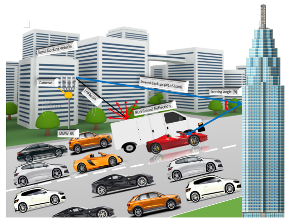
(b) The proposed scenario involves steering both LoS and NLoS with (NLoS) backup.
