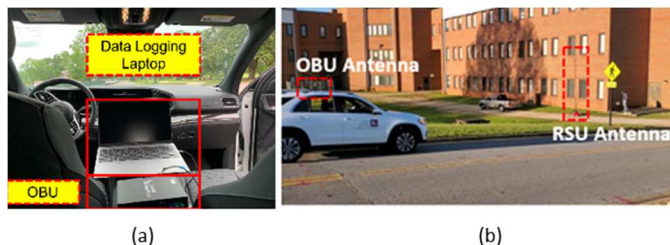
Fig. 1. Setup of real-world test; (a) OBU inside the test vehicle, (b) OBU and RSU antenna placement utilized in the test
