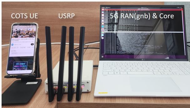
Fig. 4. Actual 5G traffic on UE(through USRP, gNodeB, 5G Core).
