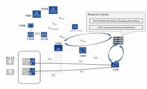
Fig. 1. Network architecture of the porposed scheme
