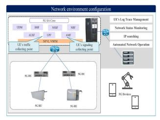
Fig. 3. Network environment cofiguration for implementation
