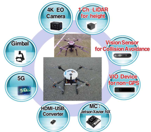
Fig. 3. The structure of the implemented drone for dedicated for facilities inspection.
