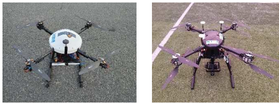
Fig. 5. The developed drones for facility safety monitoring
