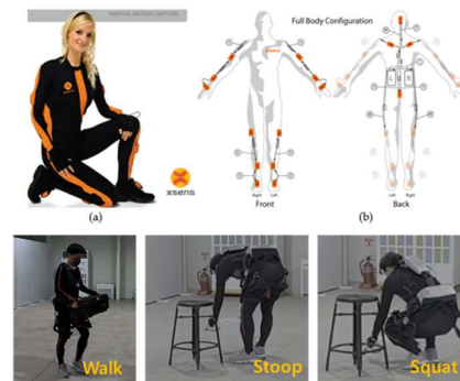
Fig. 2. Xsens MVN device-based motion data collection
